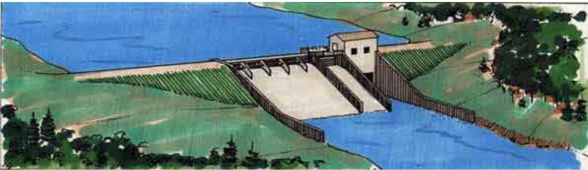
**Gated Dam with Powerhouse and Tainter Gate Spillway**
