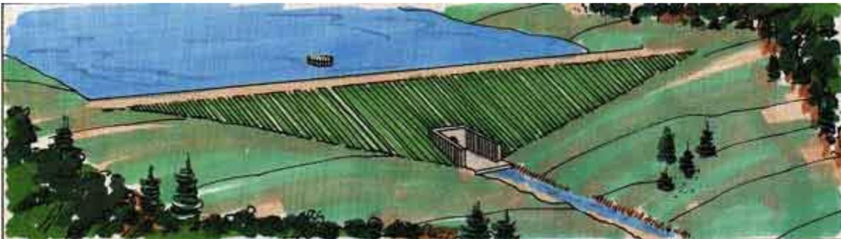
**Earth Embankment with Drop Inlet**
